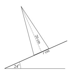
A uniform solid cone has vertical height 20 cm and base radius r cm. It is placed with its axis vertical on a rough horizontal plane. The plane is slowly tilted until the cone topples when the angle of inclination is  $24^{\circ}$  (see diagram).
