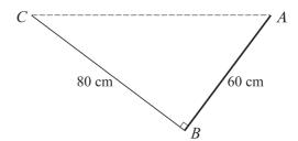
A uniform rod AB of length 60 cm and weight 15 N is freely suspended from its end A. The end B of the rod is attached to a light inextensible string of length 80 cm whose other end is fixed to a point C which is at the same horizontal level as A. The rod is in equilibrium with the string at right angles to the rod (see diagram).
