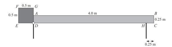
A barrier is modelled as a uniform rectangular plank of wood, ABCD, rigidly joined to a uniform square metal plate, DEFG. The plank of wood has mass 50 kg and dimensions 4.0 m by 0.25 m. The metal plate has mass 80 kg and side 0.5 m. The plank and plate are joined in such a way that CDE is a straight line (see diagram). The barrier is smoothly pivoted at the point D. In the closed position, the barrier rests on a thin post at H. The distance CH is 0.25 m.
