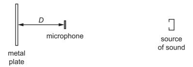
Sound of the unknown frequency is reflected back from a metal plate. A microphone placed at a distance D from the metal plate detects the sound intensity. A minimum intensity is detected with  $D = 12.0 \,\mathrm{cm}$ . The plate is moved further away from the microphone until the next minimum is detected with  $D = 15.0 \,\mathrm{cm}$ .
