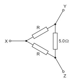
The resistance between Y and Z is found to be  $2.5 \Omega$ .
