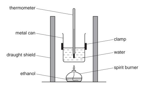
The ethanol in the spirit burner was burned to heat a measured mass of water in the metal can. The student recorded the initial and final mass of ethanol and the initial and final temperature of the water for each experiment.
