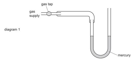
When the gas supply is turned on, the mercury in the tube connected to the supply falls by 40 mm and the mercury in the tube open to the atmosphere rises by 40 mm, as shown in diagram 2.
