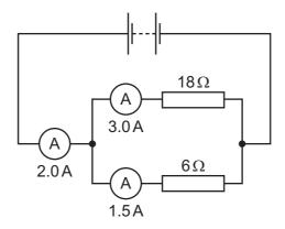
How do we know that at least one of the ammeters must be faulty?
