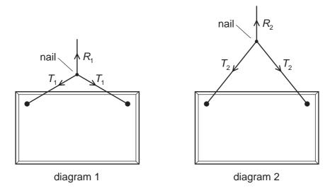
In both cases, a string is attached to the same points on the picture and looped symmetrically over a nail in a wall. The forces shown are those that act on the nail.
