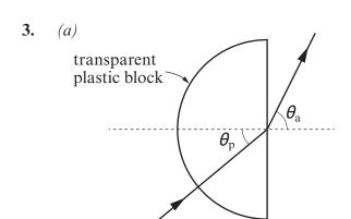
A student traces the path of a narrow beam of light through a transparent plastic block, and measures the angles  $\theta_a$  and  $\theta_p$  (see diagram). She repeats the measurements for various chosen values of  $\theta_p$ , and her results are plotted below.
