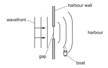
What is the name of this curving effect, and how can the gap be changed so that the wavefronts do not reach the boat?
