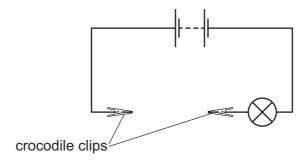
Four cylinders W, X, Y and Z are made of the same metal but have different dimensions. The cylinders are connected in turn, by their ends, between the crocodile clips. The diagrams of the cylinders are all drawn to the same scale.
