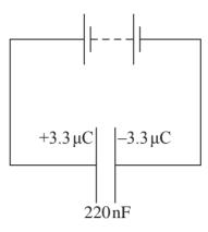
(a) Calculate the e.m.f. of the battery and the energy stored in the charged capacitor.
