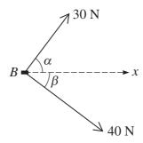
A block B lies on a rough horizontal plane. Horizontal forces of magnitudes 30 N and 40 N, making angles of  $\alpha$  and  $\beta$  respectively with the x-direction, act on B as shown in the diagram, and B is moving in the x-direction with constant speed. It is given that  $\cos \alpha = 0.6$  and  $\cos \beta = 0.8$ .
