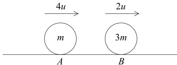
The sphere  $A$  collides directly with sphere  $B$ . The coefficient of restitution between  $A$  and  $B$  is  $e$ .
