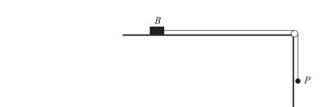
A block *B* of mass 0.4 kg and a particle *P* of mass 0.3 kg are connected by a light inextensible string. The string passes over a smooth pulley at the edge of a rough horizontal table. *B* is in contact with the table and the part of the string between *B* and the pulley is horizontal. *P* hangs freely below the pulley (see diagram).
