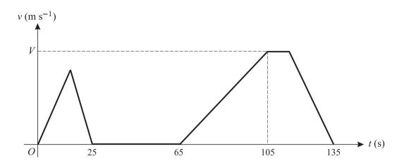
The diagram shows the (t, v) graph for the motion of a hoist used to deliver materials to different levels at a building site. The hoist moves vertically. The graph consists of straight line segments. In the first stage the hoist travels upwards from ground level for 25 s, coming to rest 8 m above ground level.
