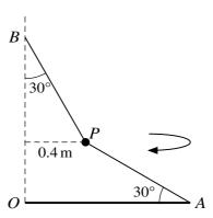
OA is a rod which rotates in a horizontal circle about a vertical axis through O. A particle P of mass 0.2 kg is attached to the mid-point of a light inextensible string. One end of the string is attached to the rod at A and the other end of the string is attached to a point B on the axis. It is given that OA = OB, angle  $OAP = \text{angle } OBP = 30^{\circ}$ , and P is 0.4 m from the axis. The rod and the particle rotate together about the axis with P in the plane OAB (see diagram).
