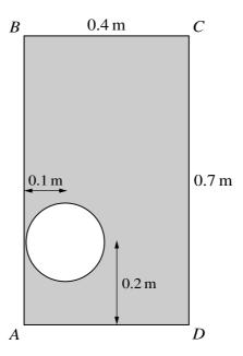
A uniform object is made by drilling a cylindrical hole through a rectangular block. The axis of the cylindrical hole is perpendicular to the cross-section ABCD through the centre of mass of the object. AB = CD = 0.7 m, BC = AD = 0.4 m, and the centre of the hole is 0.1 m from AB and 0.2 m from AD (see diagram). The hole has a cross-section of area 0.03 m<sup>2</sup>.
