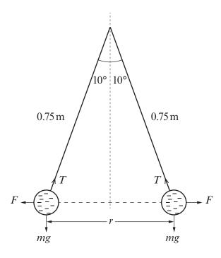
The weight mg of each balloon, the electrostatic forces F acting on each balloon and the tensions T in the strings are shown in the diagram.
