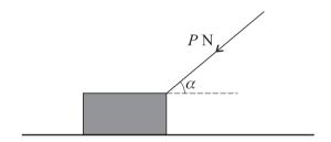
When a force of magnitude P N acts downwards on the block at an angle  $\alpha$  to the horizontal, as shown in the diagram, the frictional force on the block has magnitude 6 N and the block is again on the point of slipping. Find
