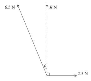
Forces of magnitudes 6.5 N and 2.5 N act at a point in the directions shown. The resultant of the two forces has magnitude R N and acts at right angles to the force of magnitude 2.5 N (see diagram).
